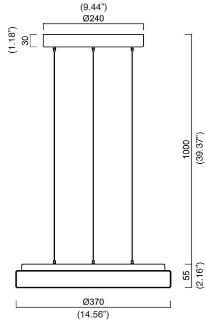
Round pendant light with shade diameter Ø370mm (14.56"). Product consists of cableless pendant opal polycarbonate shade. Shade is fixed by two-step clamp holders. Suitable for indoor use.
