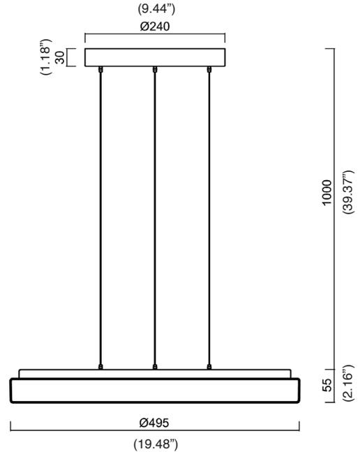
Round pendant light with shade diameter Ø495mm (19.48"). Product consists of cableless pendant opal polycarbonate shade. Shade is fixed by two-step clamp holders. Suitable for indoor use.
