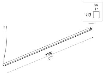
Lighting modular system with direct light. Aluminum structure in matt white, embossed black or gold finish. Linear profiles with opal polycarbonate, and round structures with opal polycarbonate diffuser. Strip LED on polycarbonate diffuser.
