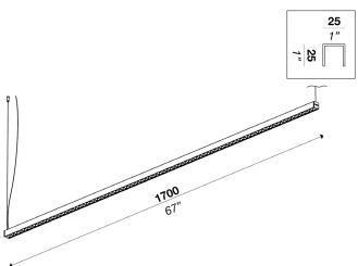
Lighting modular system with direct light. Aluminum structure in matt white, embossed black or brass finish. Linear profiles with dark light optic diffuser, and round structures with opal polycarbonate diffuser. LED module on dark light optic diffuser.
