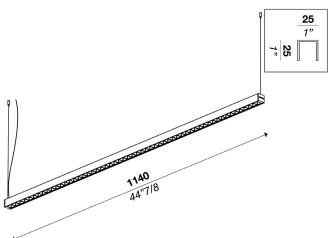
Lighting modular system with direct light. Aluminum structure in matt white, embossed black or brass finish. Linear profiles with dark light optic diffuser, and round structures with opal polycarbonate diffuser. LED module on dark light optic diffuser.
