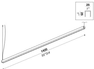
Lighting modular system with direct light. Aluminum structure in matt white, embossed black or gold finish. Linear profiles with opal polycarbonate, and round structures with opal polycarbonate diffuser. Strip LED on polycarbonate diffuser.
