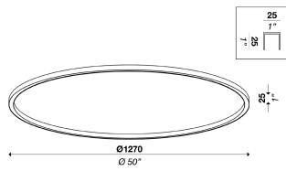
Lighting modular system with direct light. Aluminum structure in matt white, embossed black or gold finish. Round configuration with opal polycarbonate, and round structures with opal polycarbonate diffuser. Strip LED on polycarbonate diffuser.
