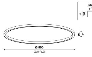
Lighting modular system with direct light. Aluminum structure in matt white, embossed black or gold finish. Round configuration with opal polycarbonate, and round structures with opal polycarbonate diffuser. Strip LED on polycarbonate diffuser.
