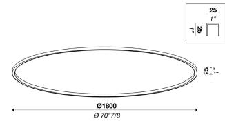
Lighting modular system with direct light. Aluminum structure in matt white, embossed black or gold finish. Round configuration with opal polycarbonate, and round structures with opal polycarbonate diffuser. Strip LED on polycarbonate diffuser.
