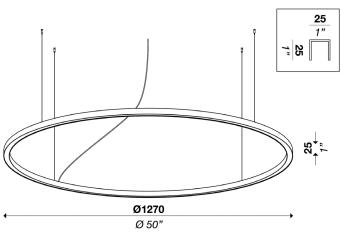
Lighting modular system with direct light. Aluminum structure in matt white, embossed black or gold finish. Round configuration with opal polycarbonate, and round structures with opal polycarbonate diffuser. Strip LED on polycarbonate diffuser.
