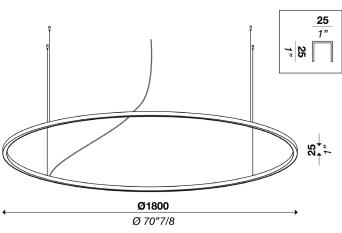
Lighting modular system with direct light. Aluminum structure in matt white, embossed black or gold finish. Round configuration with opal polycarbonate, and round structures with opal polycarbonate diffuser. Strip LED on polycarbonate diffuser.
