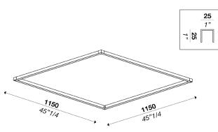
Lighting modular system with direct light. Aluminum structure in matt white, embossed black or gold finish. Linear profiles with opal polycarbonate, and round structures with opal polycarbonate diffuser. Strip LED on polycarbonate diffuser.
