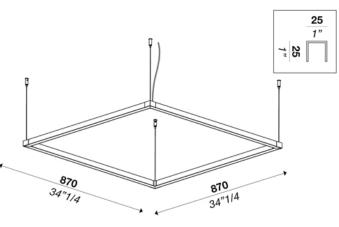
Lighting modular system with direct light. Aluminum structure in matt white, embossed black or gold finish. Linear profiles with opal polycarbonate, and round structures with opal polycarbonate diffuser. Strip LED on polycarbonate diffuser.
