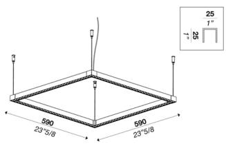
Lighting modular system with direct light. Aluminum structure in matt white, embossed black or brass finish. Linear profiles with dark light optic diffuser, and round structures with opal polycarbonate diffuser. LED module on dark light optic diffuser.
