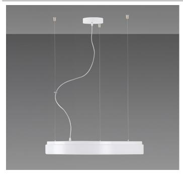
Cylindrical pendant light with shade diameter Ø650mm (25.59"). Product consists of powder-coated metal base and PMMA shade. Shade is fixed by two-step clamp holders. Suitable for indoor use.
