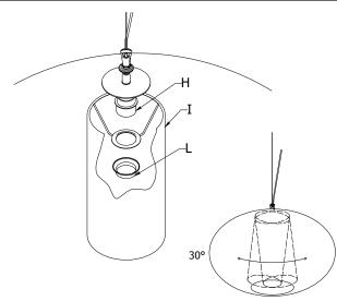
The inner lampshade of all set and models is placed on an articulated joint which allow a slight inclination in all direction to have a perfect balance of the swinging lamp.
