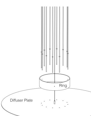
4. Pass the steel wire through the ring and insert the wire through the cable gripper. Adjust the length of the steel wire to adjust the height of the diffuser plate as desired.
