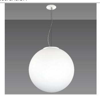
Spherical pendant light with shade diameter Ø600mm (23.62") Product consists of wire pendant and PMMA matt shade. Shade is fixed by steel hanger. Suitable for indoor use.
