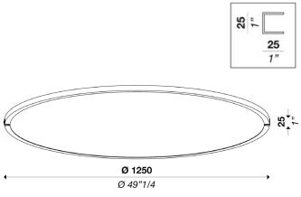
Ceiling lamp Ø 1250mm (49"1/4) with direct light. Aluminum structure matt white, black or brass coated. Opal membrane diffuser. Strip LED.
