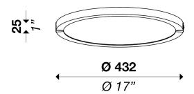
Ceiling lamp Ø 430mm (17") with direct light. Aluminum structure matt white, black or brass coated. Opal membrane diffuser. Strip LED.
