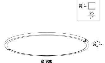
Ceiling lamp  $\emptyset$  900mm (35"1/2) with direct light. Aluminum structure matt white, black or brass coated. Opal membrane diffuser. Strip LED.
