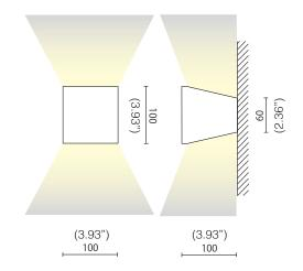
Characterized by the symmetrical cuts, Mia is a dou-ble emission wall lamp made from epoxy polyester powder coated aluminium and it is equipped with Chip On Board technology high efficiency LED light sources and driver. Its degree of protection against the penetration of dust, solid objects and liquids is IP20.
