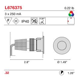
Recessed spotlight in nickel matte finish or white painted. Heatsink included. Available in round or square version. Installation with or without junction box and on metal false celling with adapter.
