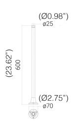
ø 25 mm (Ø 0.98") Ø 70 mm (Ø2.75") H 600 mm (23.62") **BOLLARD**
