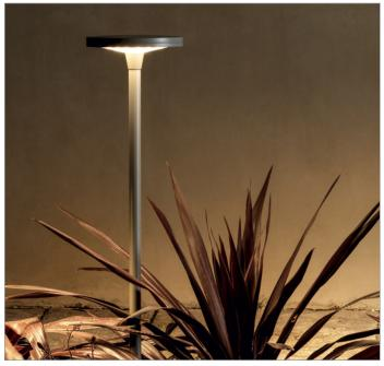
Outdoor lighting fixture for installation on a stem Dissipating upper disc in low copper content die-cast aluminum; the particular convex shape avoids water stagnation. Photo-etched polycarbonate diffuser to prevent horizontal glare and to grant high output downwards.
