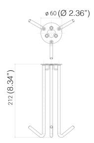
Stainless steel plate with ground anchoring set
