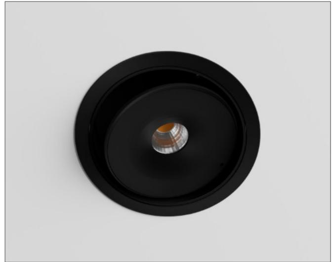
R93 is a small, movable spotlight in the shape of a disk. Thanks to a durable mechanism, we can tilt the reflector in different directions. Another advantage of this luminaire is very shallow installation – only 5.5cm (2.16”). High colour rendering index (CRI98) and a recessed light source guarantee visual comfort, while protecting one’s eyes from an unpleasant glare.
