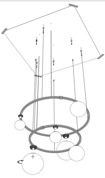
4: tape the template firmly to the ceiling (with the drawing facing the ceiling) in the desired position. Use centermark on the template if necessary
