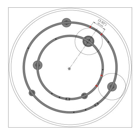
3: FOR MULTIPLE BOUNCE CONCENTRIC INSTALLATION ONLY: check where the biggest globes will be (indicated on the LED with a sticker "L") and avoid steelcables, powercables on the other rings in the areas between the red lines, as shown in the illustration.
