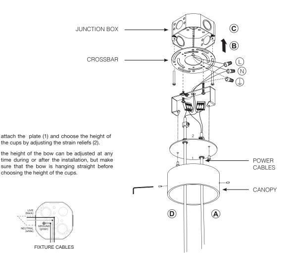
General installation and maintenance directives concerning factory guarantee. Connecting and testing the lamps must always happen by an acknowledged electrician according to the locally applying regulations on electric installations. Do not place on a flammable surface.
