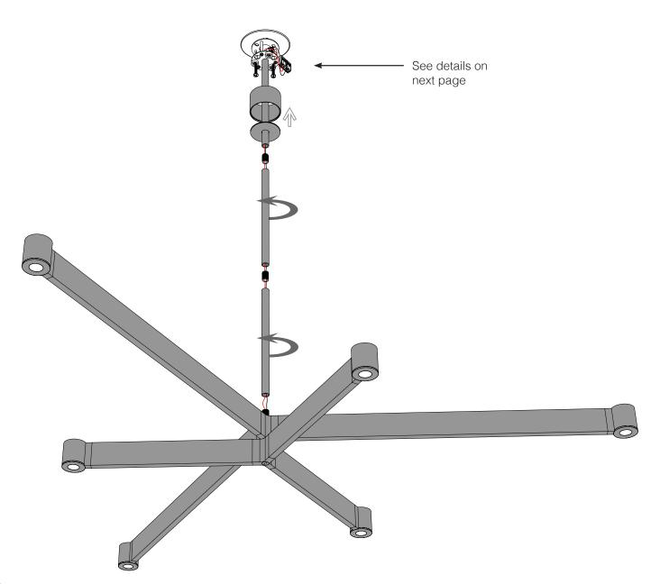
Place the components on a soft surface. fit the wires through the rods and tighten. \* grid globe: do not attach the globes to the profiles yet.
