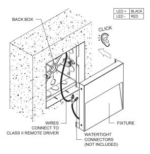
Make wire connections to the class II remote driver using watertight connectors (not included). Push the fixture in the back box untilt it clicks in place.
