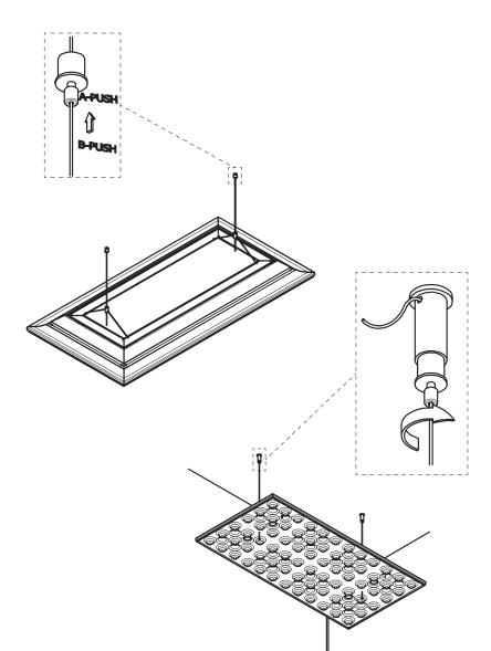
6 Adjust the cable length, and cut the rest.
