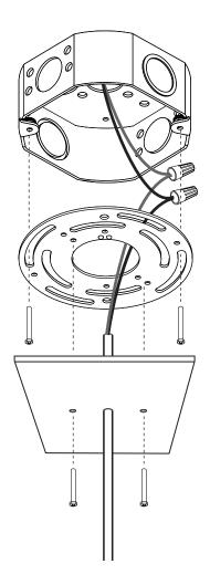
5 Install the aricraftcable and connector to the holes.
