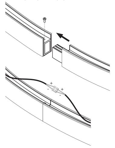
MAKE WIRING CONNECTIONS BETWEEN THE TWO SECTIONS
